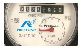
**Neptune T-10:** To check for leaks using this meter, use the red triangle. If the triangle is moving, there is water flowing through the meter.
